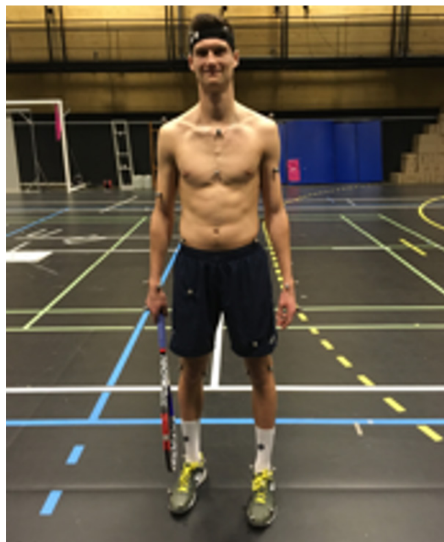
Figure 3. Player and racquet equipped with reflective body markers.
